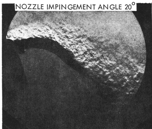
Figure 11. USB Turbulent Flow Schlieren Photographs
